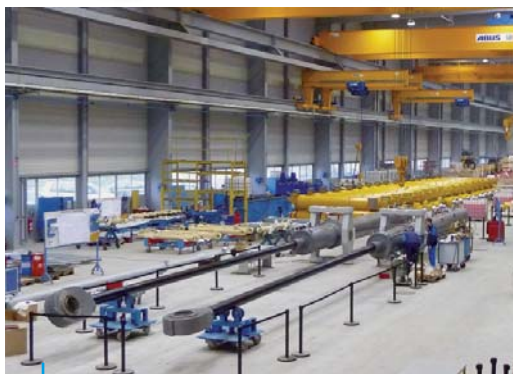
Chatou Dam (France) Radial Gate Cylinders 670 x 220, Stroke 9 250 mm Rods in KERADOUCE® coating.
