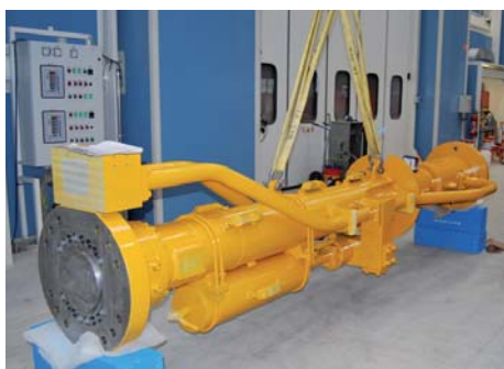
Hydraulic Pump for wave energy DA 270 x 170, Stroke 3 000 mm
