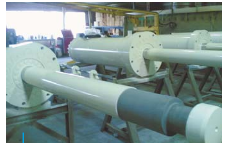
20 Cilindros tensionadores com transdutor 20 Tensioner Cylinders with Transducer
