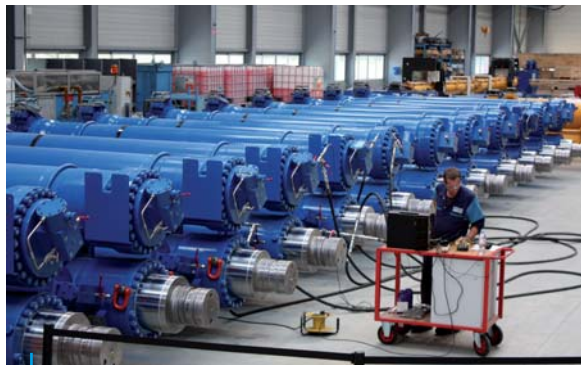
12 Wireline Riser Tensioners 280 Kips DA 555 x 480, Stroke 3 810 mm + HP accumulator dia. 580, Stroke 3 810 mm ; 1 050 liters + LP accumulator 320 liters
