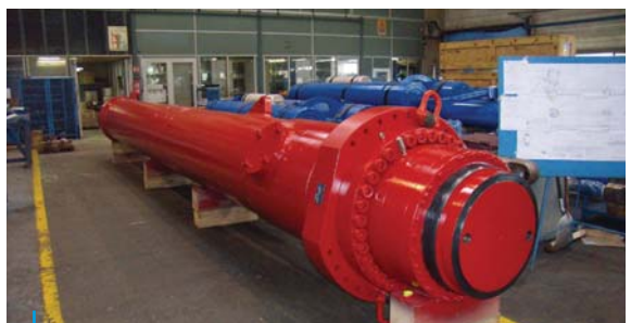
Crown Mounted Compensator Cylinder DA 820 x 720, Stroke 7 650 mm
