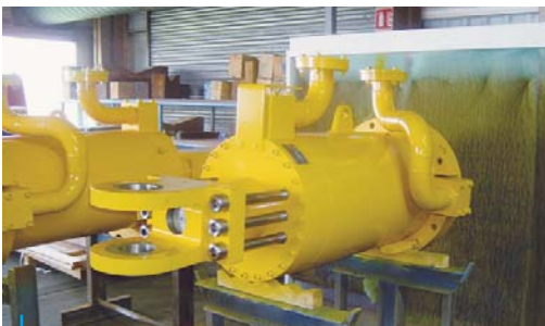
Projeto Kelsey (Manitoba/Canadá) 10 Servomotores 560 x 160, Curso 686 mm Project Kelsey (Manitoba/Canada) 10 Servomotors 560 x 160, Stroke 686 mm
