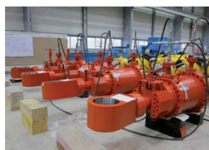
Mica Project (Canada) 4 Servomotors DA 600 x 260, Stroke 423 mm
