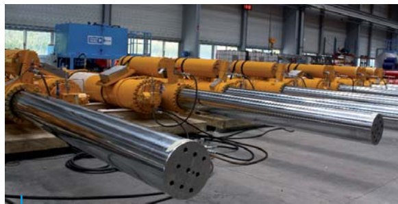
12 Wireline Riser Tensioner Cylinders 250 Kips DA 540 x 480, Stroke 3 810 mm + HP accumulator dia. 580 mm, Stroke 3 710 mm ; 980 Liters + LP accumulator dia. 304 mm, Stroke 3 450 mm ; 250 Liters
