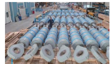
100 Hydraulic Cylinders for offshore wind turbines DA 650 x 320, Stroke 2 300 mm
