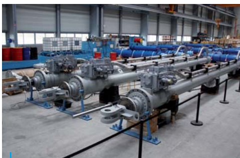
La Sarcelle Dam (Canada/Quebec) Vertical Gate Cylinders 360 x 190, Stroke 10 900 mm Rods in KERADOUCE® coating
