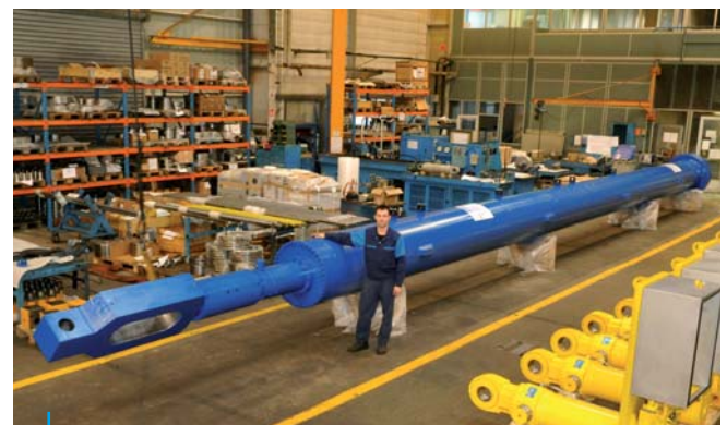
Boguchanskaya Dam (Russia 2009) Douce-Hydro has designed, manufactured, and supplied for the largest hydro power scheme under construction in Russia: 10 DA Hydraulic Cylinders 710 mm x 250 mm, Stroke 15 000 mm with KERADOUCE® coating and dual SMIK® Integrated Measuring System + hydraulic power units and control panels.
