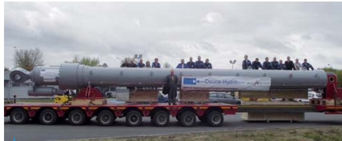
2 Hydraulic Cylinders with KERALOCK® Locking System DA 900 x 600, Stroke 12 740 mm -Force applied: 9 000 kN For J-Lay tower application
