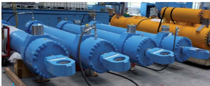
32 holder tilt Hydraulic Cylinders SA 410 x 200, Stroke 3 831 mm
