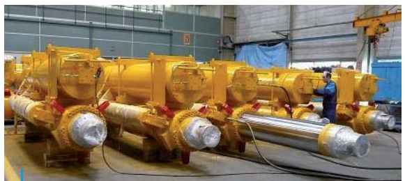
10 Wireline Riser Tensioner Cylinders 250 Kips DA 540 x 480, Stroke 3 810 mm + HP accumulator dia. 580 mm, Stroke 3 710 mm ; 980 Liters + LP accumulator dia. 304 mm, Stroke 3 450 mm ; 250 Liters
